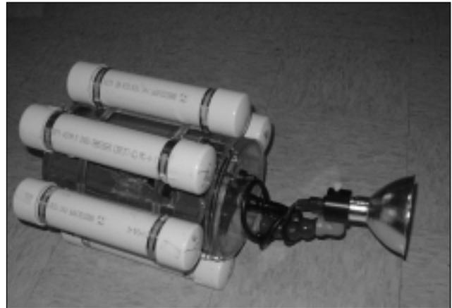
Think HID is the only way to get "Big Light"? A 250 watt halogen video light, by Mike Griffin, using 4 - 7Ah/12v batteries. The PVC tubes are for buoyancy.
