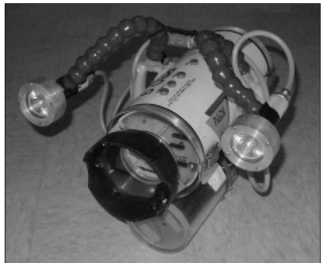
Commercial housing with homebuilt light arms and battery canister.
